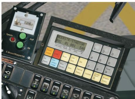
The control panel (left on the picture) and the IBIS device.
