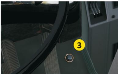
Right next to the accelerator pedal is the footswitch for the cut-off-cylinder
