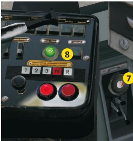
The handle (7) switches on the circulation pump of the heating circuit and opens/ closes the water valve to the radiators. Only when the handle is opened, the auxiliary heating (8) can be switched on.
