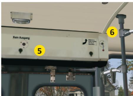
Beneath the entrance light the lock for the door wing blocking is visible. Click on it to block the rear wing of the front door. To the right you can will find the functional emergency valve to switch the door to manual operation.
